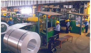
Fig. 6.3: Strip coasting mill at smelter of NALCO
