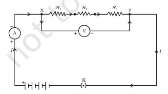
Figure 11.6 Resistors in series
