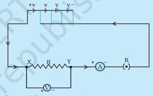
Figure 11.2 Electric circuit for studying Ohm's law
