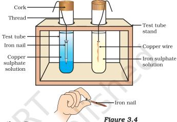
**Figure 3.4**Reaction of metals with salt solutions
