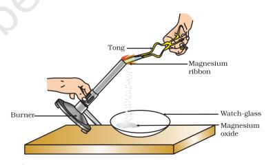
**Figure 1.1**Burning of a magnesium ribbon in air and collection of magnesium oxide in a watch-glass
