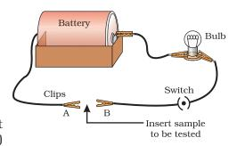
**Figure 3.2**Metals are good conductors of electricity.
