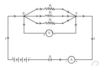
Figure 11.7 Resistors in parallel
