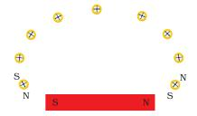
**Figure 12.3**Drawing a magnetic field line with the help of a compass needle
