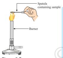
**Figure 3.7** Heating a salt sample on a spatula
