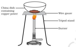
**Figure 1.10**Oxidation of copper to copper oxide
