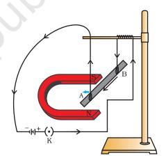
Figure 12.12 A current-carrying rod, AB, experiences a force perpendicular to its length and the magnetic field. Support for the magnet is not shown here, for simplicity.
