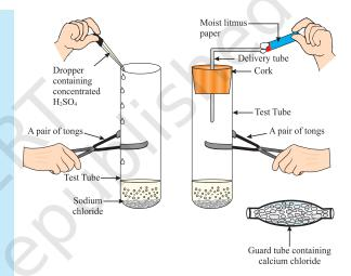
Figure 2.4 Preparation of HCl gas
