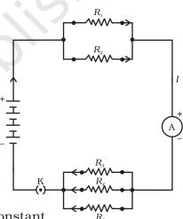
**Figure 11.12**An electric circuit showing the combination of series and parallel resistors
