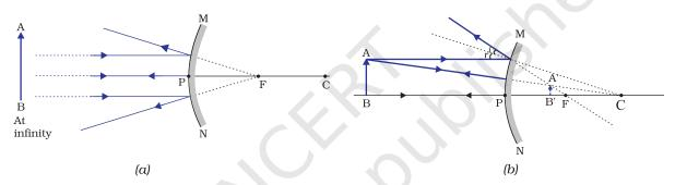
Figure 9.8 Formation of image by a convex mirror
