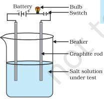
**Figure 3.8**Testing the conductivity of a salt solution
