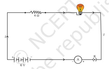
Figure 11.9 An electric lamp connected in series with a resistor of 4  $\Omega$  to a 6 V battery
