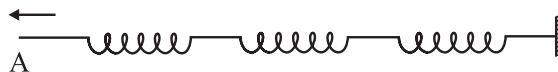
Fig. 14.1 A collection of springs connected to each other. The end A is pulled suddenly generating a disturbance, which then propagates to the other end.
